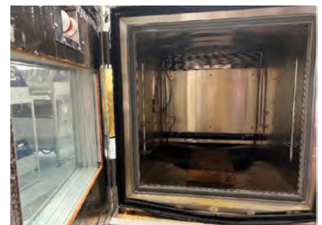
Cleveland Condensation Chamber
